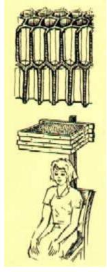
honeycombs. The cap could be made of cardboard, veneer, or better still, of tin plate with tightly sealed seams.
