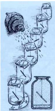
Here they are in the drawing: sealed vessels with straws and burnt twigs, drawing coals-suspended on spider web threads. There is some water at the bottom to counter static electricity hindering experiments in dry air.
