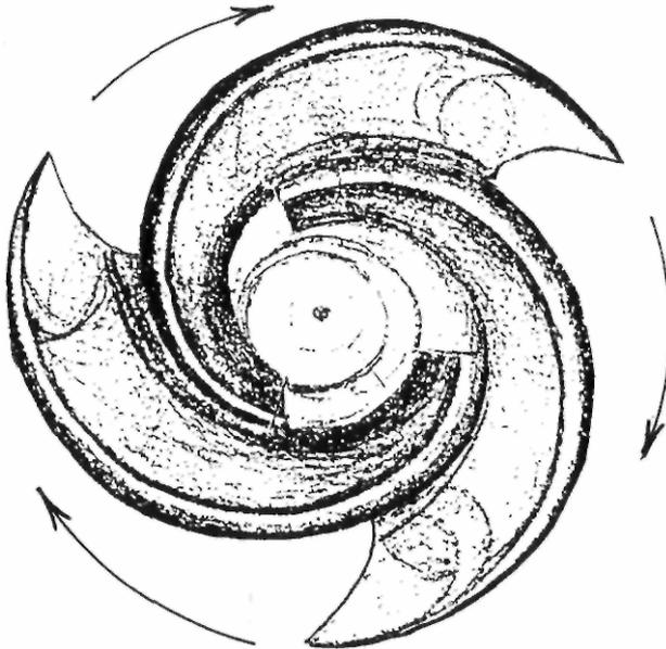
Fig. 11: 3-blade Bio-impeller
